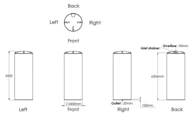
Supplied: Ball valve, overflow strainer
